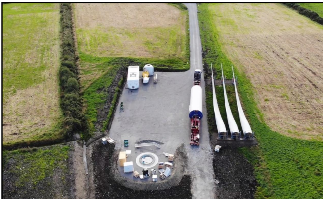
Figure 3-6: Typical Finished Hardstand
